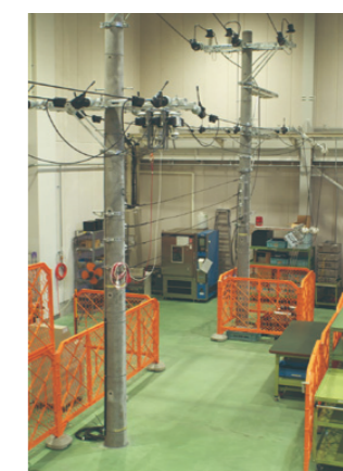
Simulated power pole for electricity distribution line
